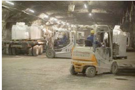
Handling of packed residues underground.
